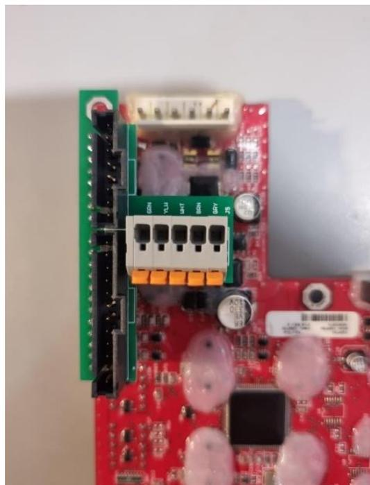
***A Fitted Adapter on Genie PCB***
