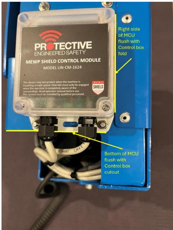
***Mounted Protective Shield Control Module***
