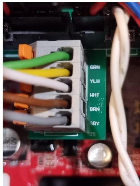
*Connecting the Relay/Power Cable*
