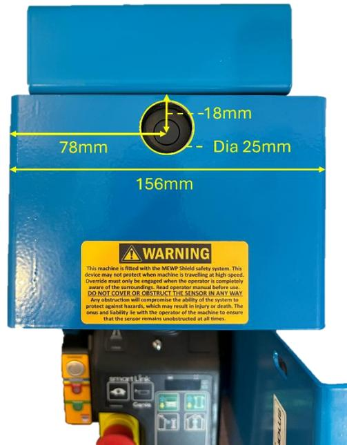
**Sensor fitted properly at its place**
