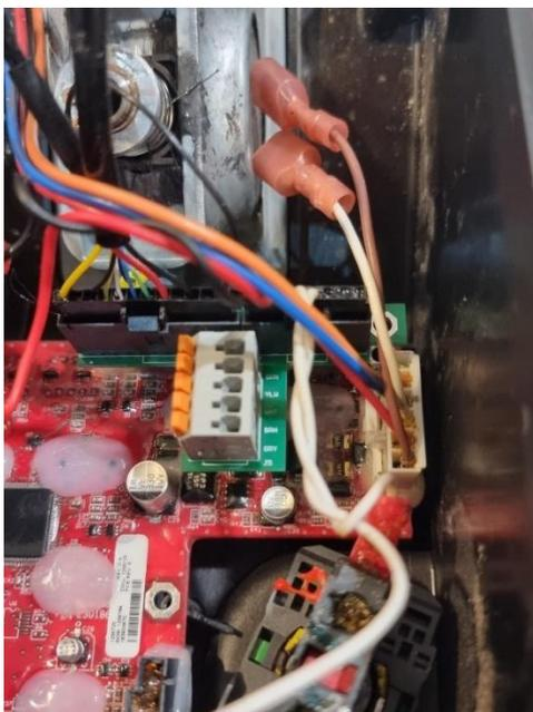
*Connecting Joystick, Buzzer/E-Stop Cables*
